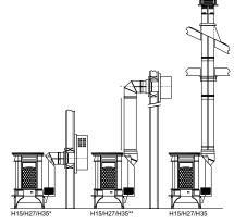
\* The H15 can be vented horizontally with the AstroCap<sup>™</sup> system. For rear vent applications, H27 and H35 require a riser vent. \*\* H35 requires minimum 1 ft. rise.
