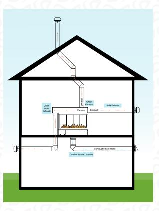
Above: Venting any direction up to 11 elbows, 110 feet and six feet down allows you to place a fireplace anywhere.
